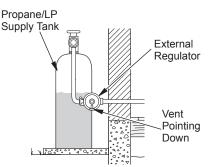
Figure 14 - External Regulator With Vent Pointing Down
